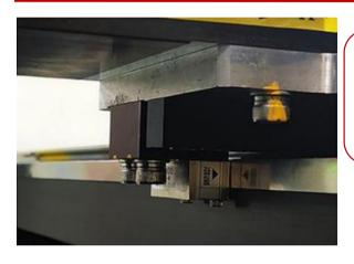
The magnetic linear encoder system real-time monitor the machine's accuracy and enables machine to correct error parameter automatically
