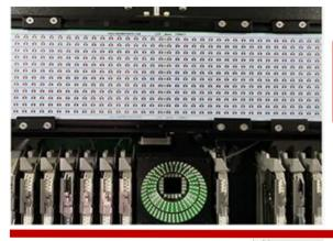
Support 1.5M LED light bar placement (optional configuration)
