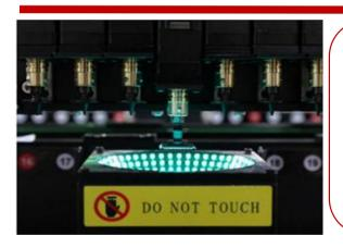
Front and rear with 2 fourth generation high speed flying camera recognition systems, US ON sensors, 28mm industrial lens, for flying shots and high accuracy recognition
