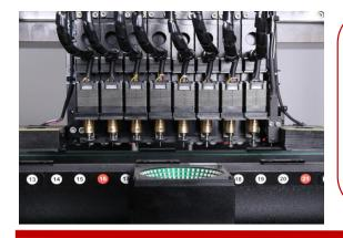
8 independent heads with fully closed-loop control system support all 8mm feeder pick up simultaneously,speed up to 13,000 CPH
