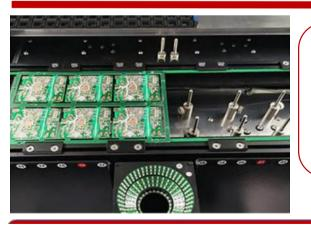
Raise PCB automatically, keeps PCB on the same surface level during placement ,ensure high accuracy
