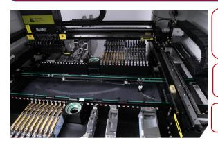
Equips double mark camera + double side high precision flying camera ensure high speed and accuracy, real speed up to 13,000 CPH. Using the real-time calculation
